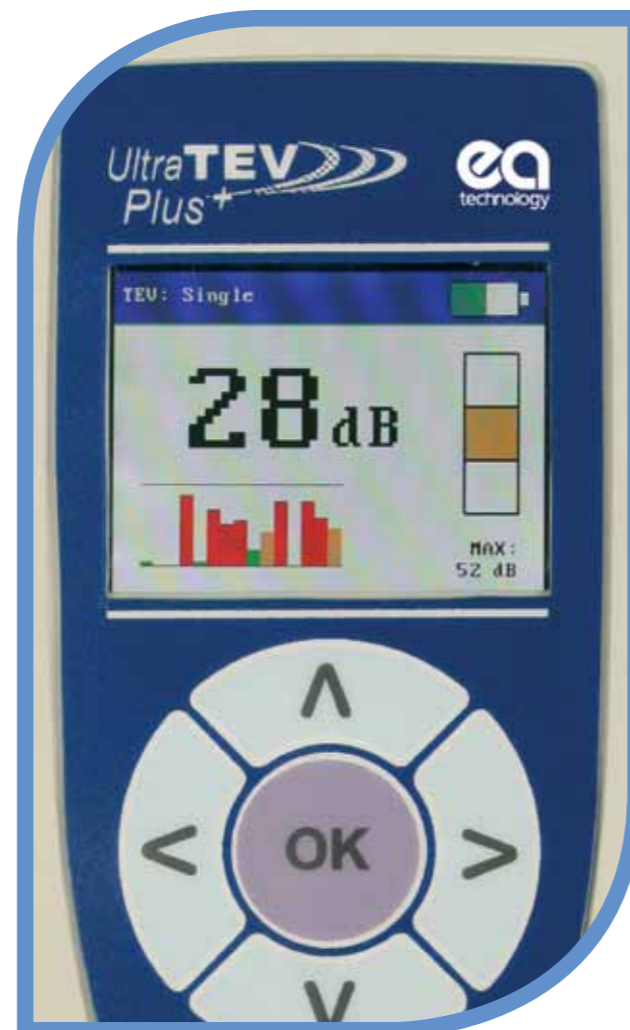
Menu-driven, multi-functional display of TEV and ultrasonic values.
